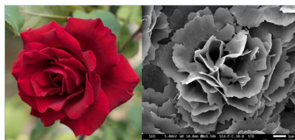
Micrograph of ZnO through controlled growth - A Nanorose [26IF0648]
